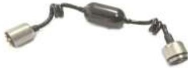
The removable sonde is located inside the spring assembly. It continually transmits a signal at 512Hz, while the camera is turned on, and can be located with any locator capable of picking up a 512Hz signal.
