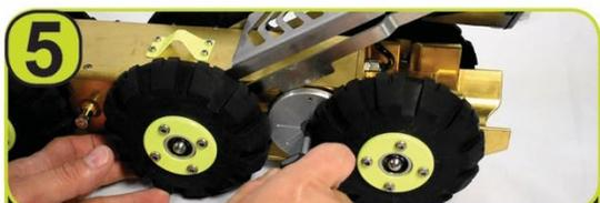
5 Set your camera height to desired pipe diameter using camera head adjustment cam.
