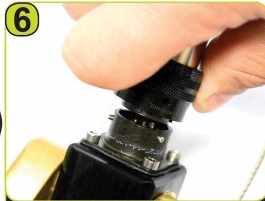
**6** Screw counter clockwise to disconnect crawler from cable.
