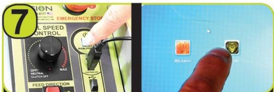
7 Press the power button on the face of the system. Select User option on boot-up screen (admin for service only).
