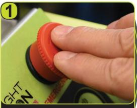
Push in the emergency stop to shut off power to the crawler.
