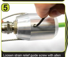
wrench and remove the cable.
